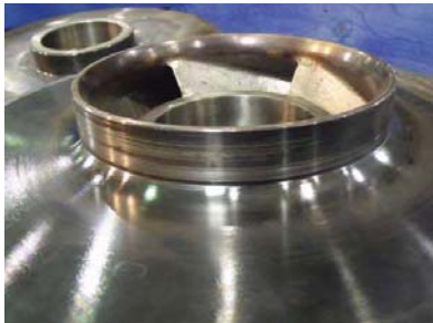
Scoring and wear on impellers. Impellers with excessive wear will require regrind and overlay of DLC coating.
