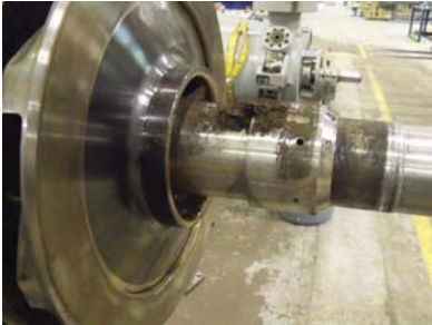
Impeller and stage casing – coker debris present.
